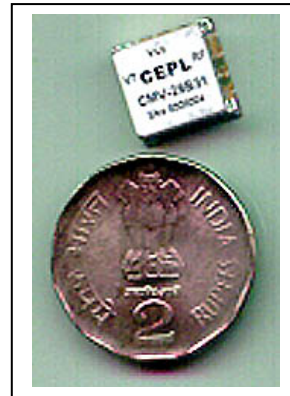
Fig 3 Photograph of the developed small foot print VCO
